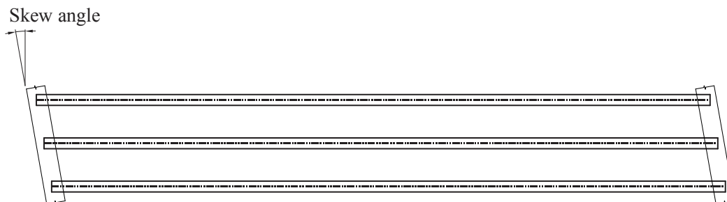
Figure 2.4 Definition of skew (top view)
